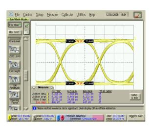
EVB Measurement Static Switch Vee: -3.3 V Output data rate: 2.5 Gb/s Data input: 300 mVpp SE
