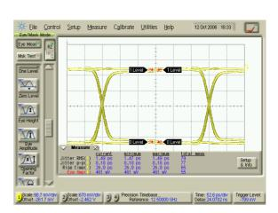
EVB Measurement Dynami4 4:1 Mux Vee: -3.3 V Output data rate: 12.5 Gb/s Data input: 300 mVpp SE
